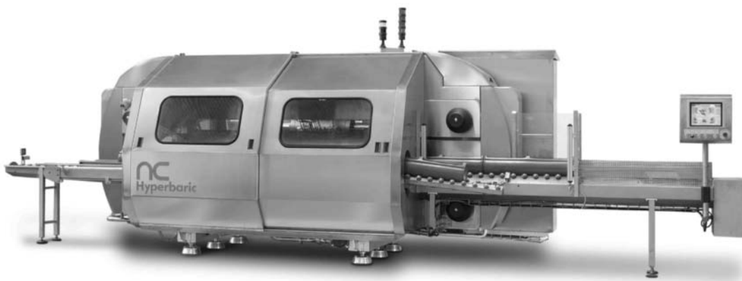
Figure 4.5. Wave 6000/55 NC Hyperbaric high-pressure-processing equipment (55-L vessel volume—maximum working pressure: 600 MPa/87,000 psi).
