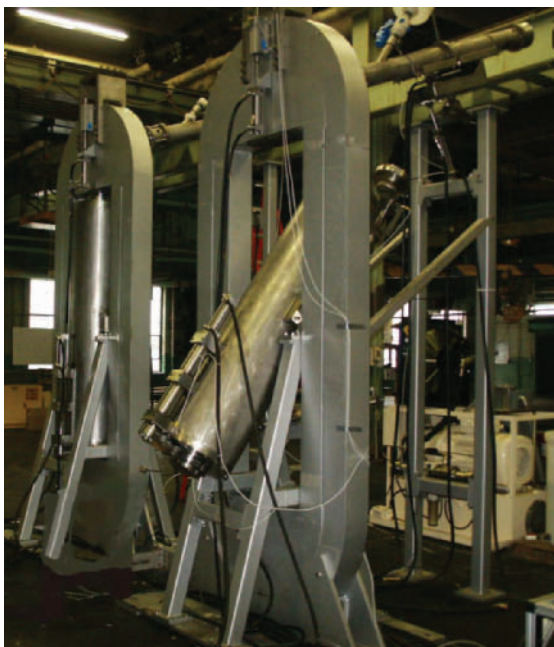
Plate 4. Pressure vessels, and their associated closure retaining yokes, can be operated at any desired angle of repose from horizontal to vertical. Units are available that tilt to receive product through the top opening, swing to a vertical position to engage a yoke during pressure treatment, then tilt to release treated product from their bottom opening. (Photo courtesy of Elmhurst.)
