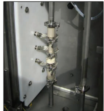
Plate 13. 16 kW continuous power ultrasound treatment system. (Courtesy of Hielscher USA, Inc.)
