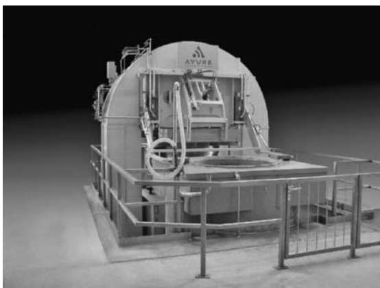
Figure 2.4. Historically, large pressure vessels have been built to operate in the vertical position and are loaded and unloaded through their top opening. (Photo courtesy of Avure.) (For color detail, see color plate section.)
