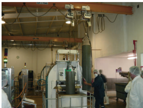
Plate 6. A second-generation yoke-based system with a 215 L volume which operates at a pressure of 600 MPa (87,000 psi). It is vertically orientated to minimize floor space. A high power pump-intensifier is located below the loading and unloading area. (Photo courtesy of Avure.)
