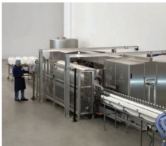
Plate 7. A third-generation 350 L volume, 600 MPa (87,000 psi) system that is capable of a 2,300 kg (5,000 pounds) per hour throughput. It is easily integrated into a horizontal product delivery subsystem. (Photo courtesy of Avure.)
