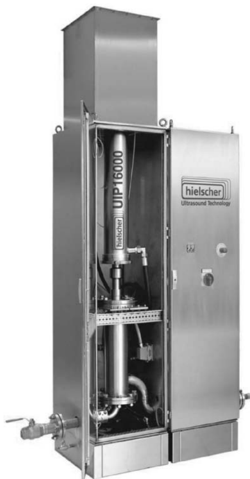
Figure 10.6. 16 kW continuous power ultrasound treatment system. (Courtesy of Hielscher USA, Inc.) (For color detail, see color plate section.)
