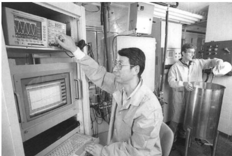
Figure 15.2. RFEF pilot plant system including fluid handling equipment, 80 kW power supply, and monitoring equipment (photograph by Peggy Greb, USDA-ARS).
