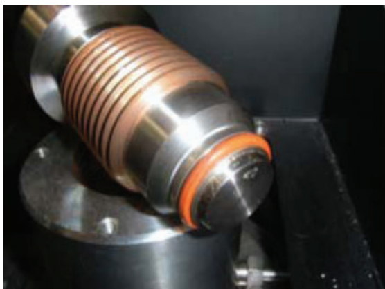
Plate 2. Typical small pressure vessels using a threaded closure. (Photo courtesy of Pressure Biosciences Inc.)
