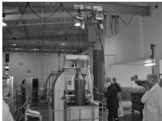
Figure 2.5. A second-generation yoke-based system with a 215 L volume which operates at a pressure of 600 MPa (87,000 psi). It is vertically orientated to minimize floor space. A high power pump-intensifier is located below the loading and unloading area. (Photo courtesy of Avure.) (For color detail, see color plate section.)
