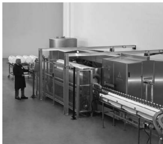
Figure 2.6. A third-generation 350 L volume, 600 MPa (87,000 psi) system that is capable of a 2,300 kg (5,000 pounds) per hour throughput. It is easily integrated into a horizontal product delivery subsystem. (Photo courtesy of Avure.) (For color detail, see color plate section.)
