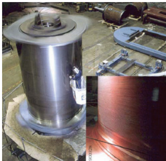
Plate 3. Wire winding can be used for both the pressure vessel and the yoke to support the end closure force. (Photo courtesy of Avure.)
