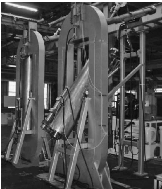
Figure 2.3. Pressure vessels, and their associated closure retaining yokes, can be operated at any desired angle of repose from horizontal to vertical. Units are available that tilt to receive product through the top opening, swing to a vertical position to engage a yoke during pressure treatment, then tilt to release treated product from their bottom opening. (Photo courtesy of Elmhurst.) (For color detail, see color plate section.)
