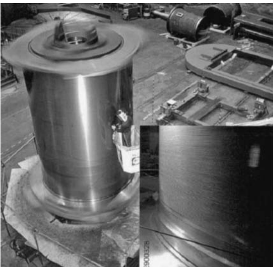
Figure 2.2. Wire winding can be used for both the pressure vessel and the yoke to support the end closure force. (Photo courtesy of Avure.) (For color detail, see color plate section.)
