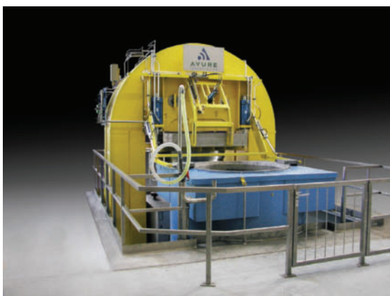
Plate 5. Historically, large pressure vessels have been built to operate in the vertical position and are loaded and unloaded through their top opening. (Photo courtesy of Avure.)
