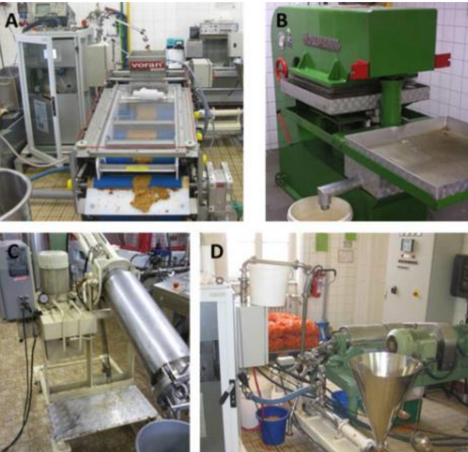
Pilot scale de-juicing systems. A) belt press; B) rack-and-cloth press; C) horizontal hydraulic filter press; D) decanter
