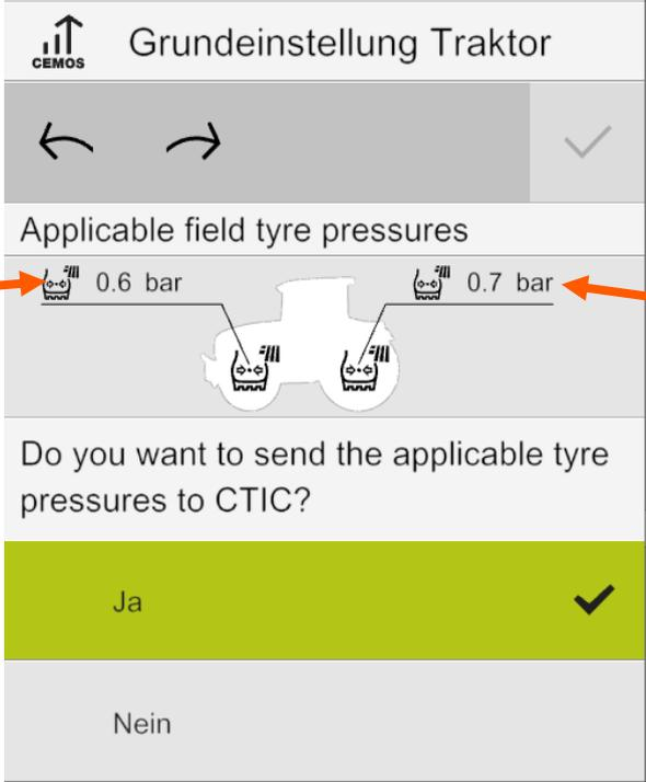
The screenshot shows the 'Grundeinstellung Traktor' (Basic Tractor Settings) menu. It features a 'CEMOS' logo and navigation arrows. The 'Applicable field tyre pressures' section displays a tractor icon with two tyre pressure values: 0.6 bar for the front axle and 0.7 bar for the rear axle. Below this is a confirmation question: 'Do you want to send the applicable tyre pressures to CTIC?'. Two options are provided: 'Ja' (Yes) with a checkmark, and 'Nein' (No).
