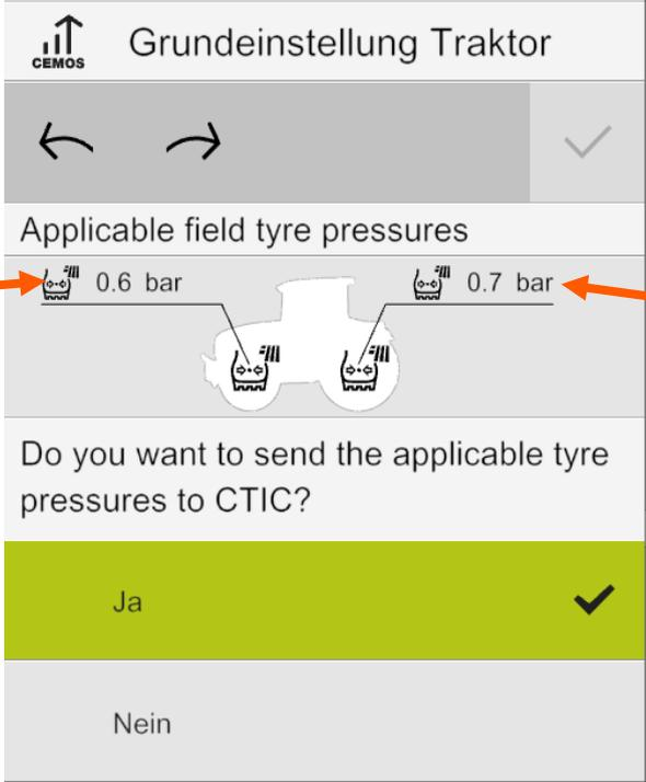
The screenshot shows the 'Grundeinstellung Traktor' (Basic tractor settings) menu. It features a back arrow, a forward arrow, and a checkmark icon. The 'Applicable field tyre pressures' section displays a tractor icon with two tyre pressure settings: 0.6 bar for the front axle and 0.7 bar for the rear axle. Below this is a confirmation question: 'Do you want to send the applicable tyre pressures to CTIC?'. Two options are provided: 'Ja' (Yes) with a checkmark, and 'Nein' (No).
