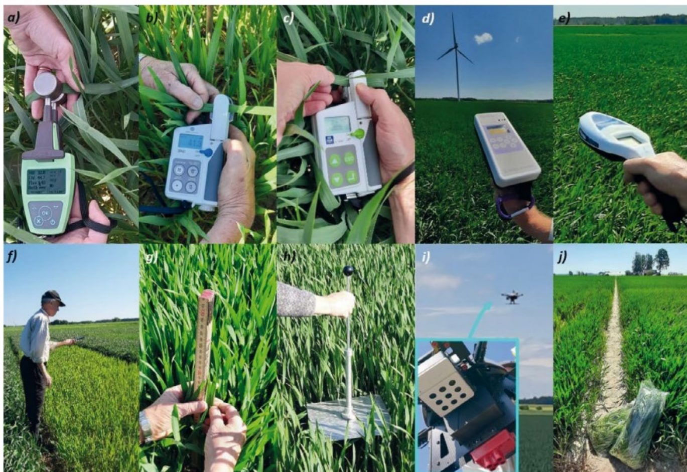
Figure 2. Equipment used in 2024. (a) Dualox, (b) SPAD, (c) N-tester, (d) RapidScan, (e) GreenSeeker, (f) Canopeo, (g) ruler, (h) platometer, (i) drones, two different sensors, and (j) cut crop samples for determination of fresh weight and N uptake.
